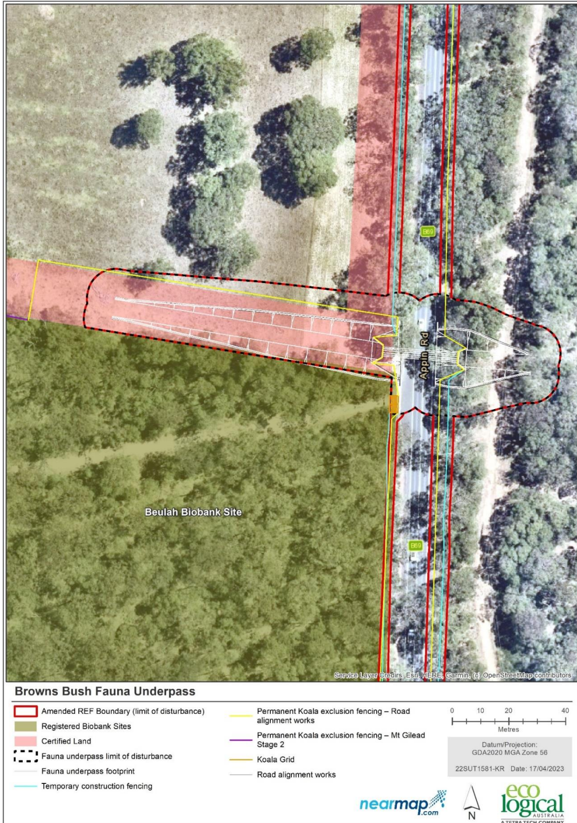
Design of Koala underpass at Browns Bush / Beulah Biobank site (part of Woodhouse Creek corridor) submitted to NSW Government as part of Appin Road upgrade.
