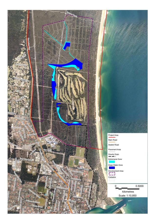
Plate 5-5 – Conceptual alignment of gravity drain
