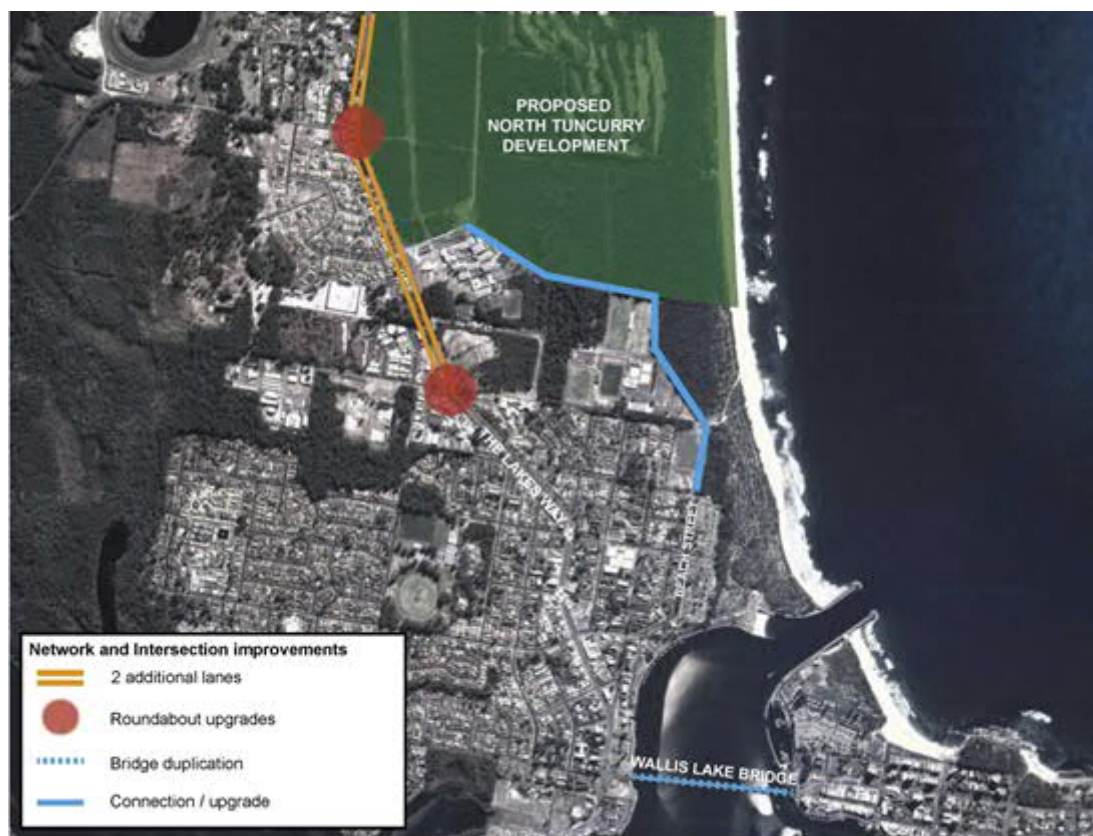
Figure 15 Road network and intersection improvements identified in the S94 Plan (for Tuncurry)
