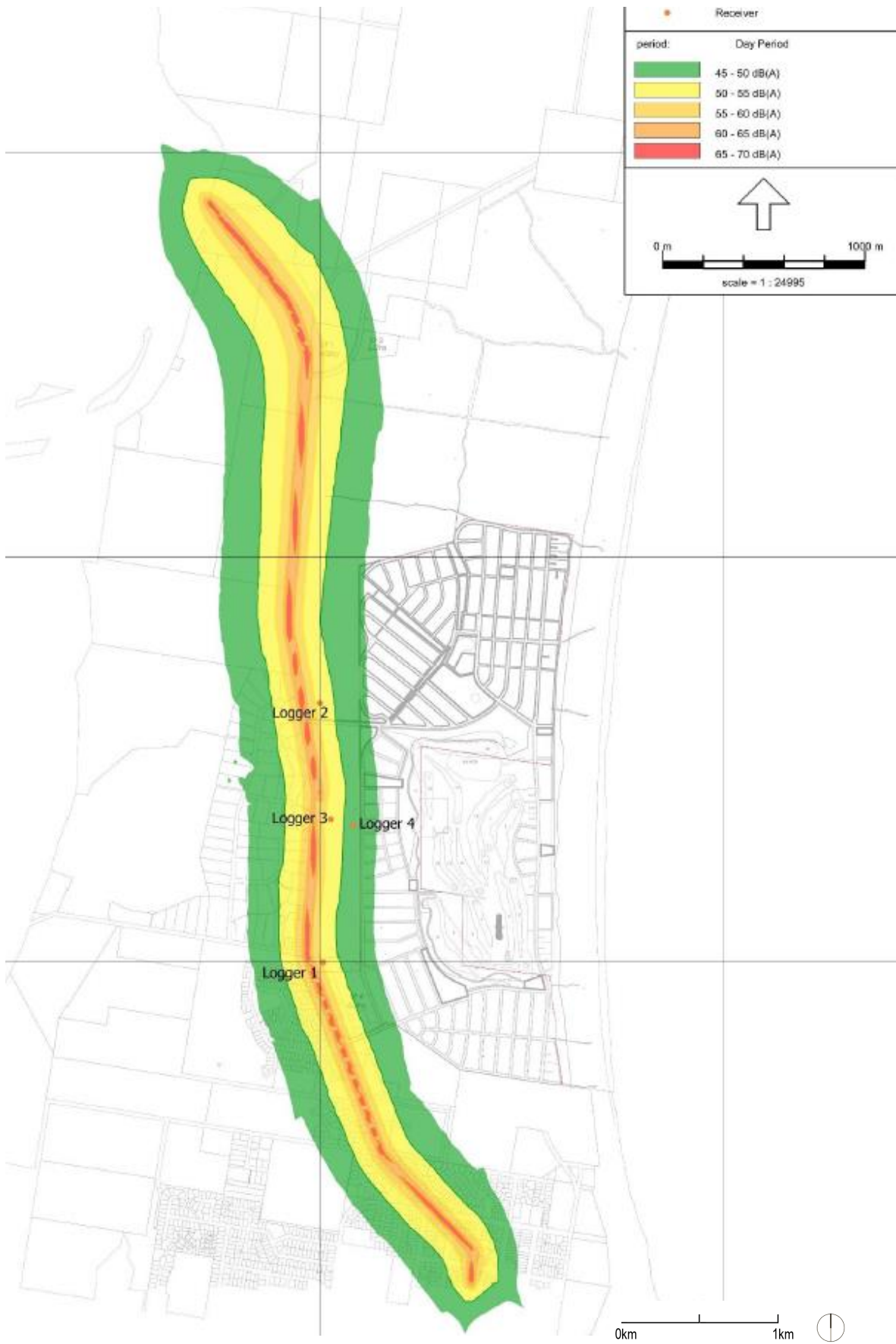
Figure 29 2023 Scenario Predicted Road Daytime Leq(15-hour) Noise Contour (no mitigation) Source: Muller Acoustic Consulting
